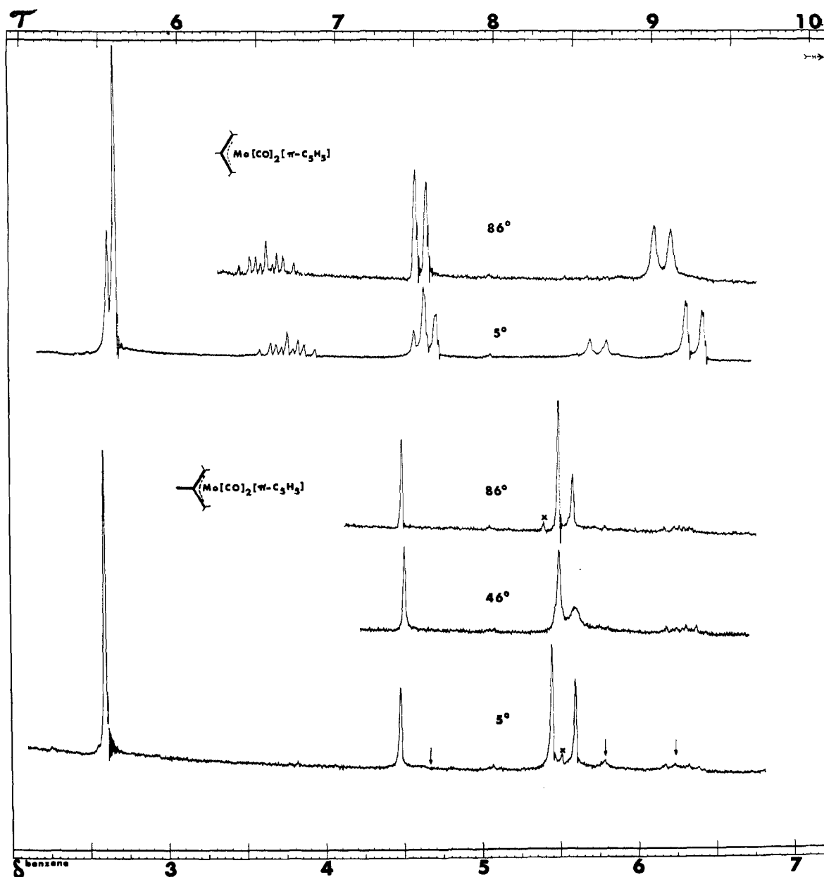
Figure 2.—The temperature dependence of the nmr spectra of \pi\text{-C}_5\text{H}_5\text{Mo}(\text{CO})_2\text{-}\pi\text{-C}_5\text{H}_5 and \pi\text{-C}_5\text{H}_4\text{Mo}(\text{CO})_2\text{-}\pi\text{-C}_5\text{H}_4 . The spectra were recorded at 100 MHz on a Varian HA-100 spectrometer operated in the frequency-sweep mode.
